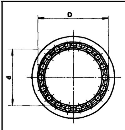
As the pm-load increases, the **stiffness** and me load carrying capacity of the **guide** system, as well as the ease of movement diminishes. If there is **insufficient pre-load**, **functional assurance will be lost**. Too much pre-load, on the other hand, will make movement **difficult** due to **high** surface pressure as the ball bearing-component is overloaded from within.
